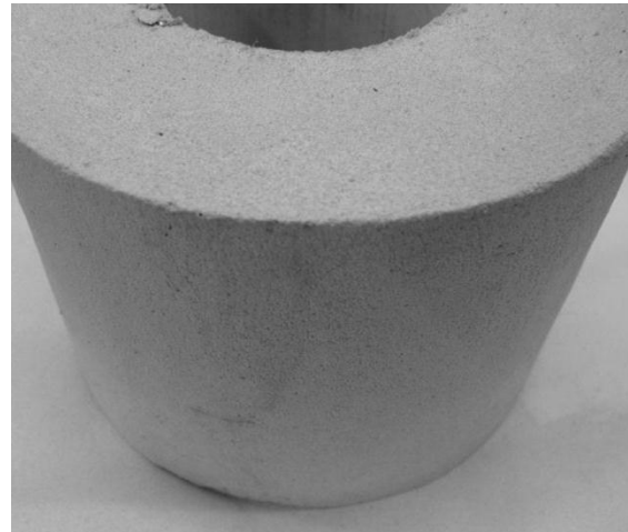
Figure 19: Specimen of Grout B after six freeze-thaw-cycles and subsequent drying.
